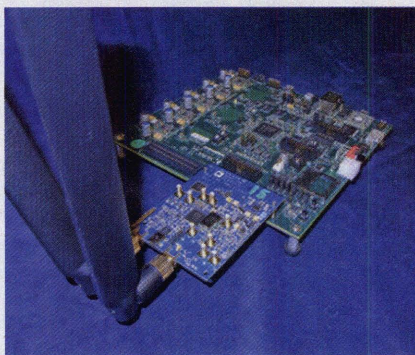
The Zynq-7000 SDR kit provides all the hardware and software for a designer to program their own commercial or military radio over wide bandwidths to 4 GHz.
