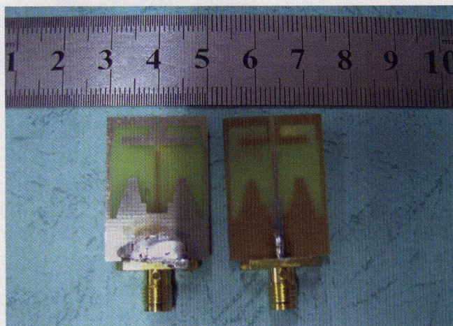
2. This photograph shows top (left) and bottom (right) views of the fabricated prototype MGS antenna.
